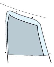
Note: When properly installed, the window can be zipped closed with Vinyl Window in place.
